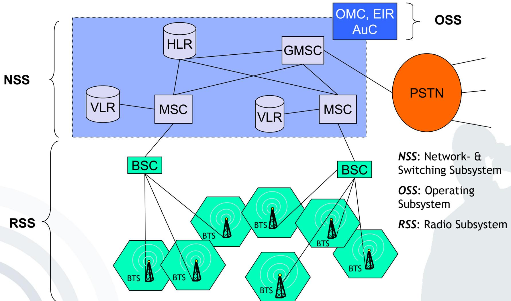
**NSS:** Network- & Switching Subsystem
