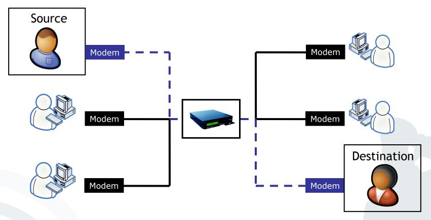
In circuit-switched networks, the communication line is used exclusively for the communicating parties (similar to the phone system, CSD and HSCSD).
